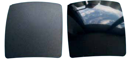
Visual effect of a typical PUD varnish containing ORGASOL® 3501 EXD NAT1 (left) vs. the uncoated glossy black ABS panel (right)
